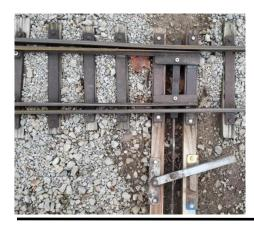
At left is a switch as found during the "walk the track" check before a run showing it stuck mid way by a small rock (at right). Make sure the handles AND the points are both sitting right.
