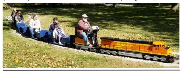
Below are pictures from the Oct 22, 2022 work day showing (L-R) Bob H, Craig B, and Bob S checking the air brake system on a blue riding car. They are using Loco 7695 to provide the pressurized air to actuate the brakes making sure the brakes work properly. Additional checks of the car, trucks, and couplers were also performed.
