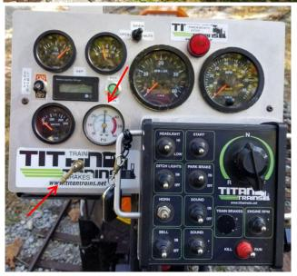
At left are the controls for 7695. The lower arrow points to the small brass pressure control handle. The upper arrow points to the air pressure gauge which shows the air pressure actually in the brake hoses on the passenger cars. It is pointing to 30 PSI which is where engineers need to set the pressure to get good braking. Rotate the brass lever clockwise to increase pressure and CCW to lower pressure.
