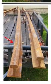
At left are rails that have been rejected due to improper bending. The bender is shown at right. It is hooked onto a rail then the center ratcheting plunger is pushed against the rail until the
